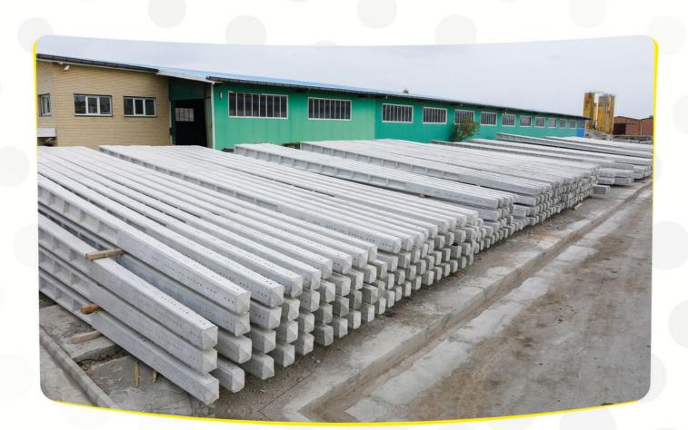
The H-type utility poles are frequently used in distribution grid networks. Through these years, "Sazehaye Novin Company" has been manufacturing these utility poles in all sizes and standard tensile strength. It is noteworthy that the company had managed to acquire all the approvals of Iran's power Generation, Distribution and Transmission company (TAVANIR).
